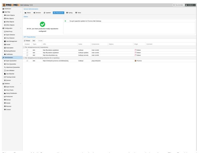
Since Proxmox Mail Gateway 7.0 you can check the repository state in the web interface. The *Dashboard* shows a high level status overview, while the separate *Repository* panel (accessible via *Administration*) shows in-depth status and list of all configured repositories.
